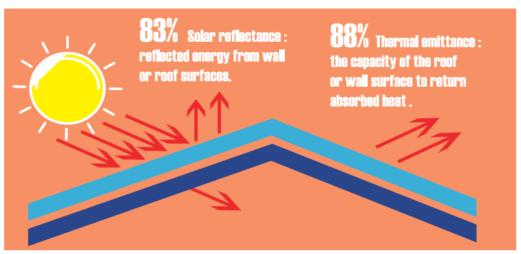
Thermal resistance R = 1,87m2K/W - Thermal transmittance : U = 0,53W/m2K - Solar reflectance index SRI : 104
